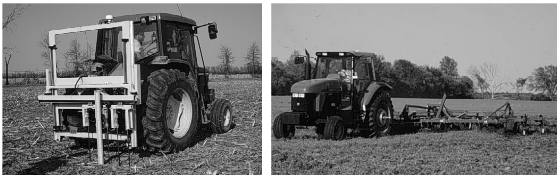
Fig. 2 Data collection for cone index (CI, left) and tillage draft (TD, right).
