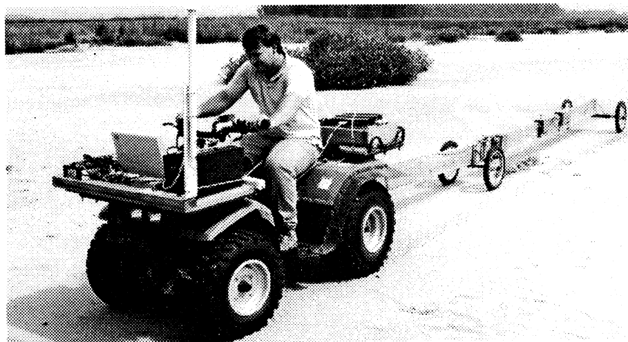
Figure 2. Mobile system for collecting EM38 and GPS data used for developing maps of sand deposition depth
