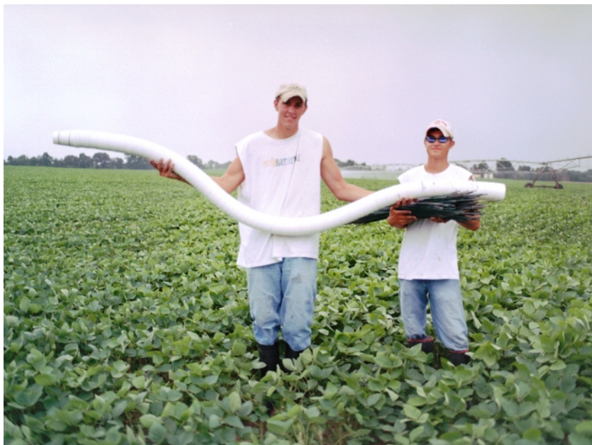
Figure 2. Technicians hold the large number of catch cans (telescoped into each other) that were used to run a single row of catch cans.
