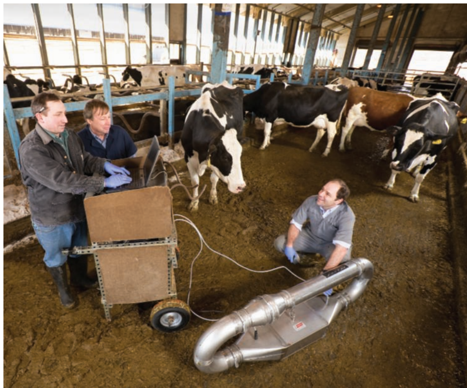
Left to right, Pennsylvania State University agricultural engineer Michael Hile, ARS agricultural engineer AI Rotz, and ARS research associate Felipe Montes use a dynamic flux chamber to measure the emission rates of gaseous compounds from manure on a dairy barn floor.
