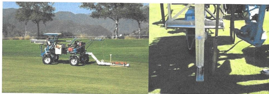
Figure 3. (a) EM 38 remote sensing field vehicle with EM38 unit positioned for EC measurements at the site. (b) Close up of soil coring instrument mounted to field vehicle.
