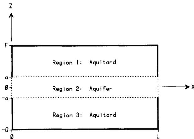
Fig. 1. Schematic diagram of the stratified aquifer-aquitard system where the bold solid and dotted lines indicate no-flow and prescribed head boundaries, respectively.
