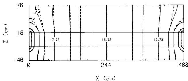
**Fig. 7. Comparison between the analytical solution (solid line) and the finite-element solution (dashed line) when the upper layer is partially saturated. The water table is described by the line 18 cm-3 cm x/L. See the text for a discussion concerning the four points marked in this figure. The contour levels are given in the text.**
