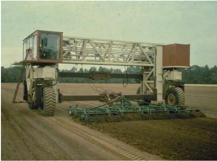
Fig. 6. Wide-frame tractive vehicle constructed at the USDA-ARS-NSDL in Auburn, AL for controlled traffic research.
