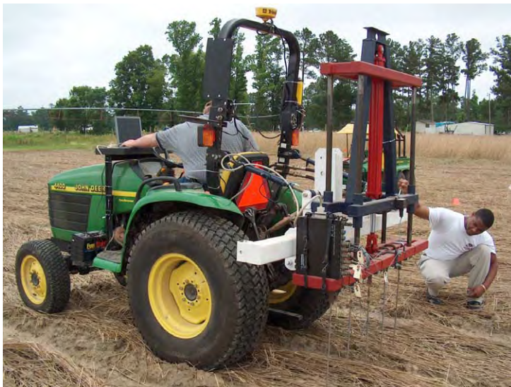
Fig. 1. Multiple-probe soil cone penetrometer system developed at the USDA-ARS National Soil Dynamics Laboratory in Auburn, AL to measure cone index across the row from a trafficked row middle to an untrafficked row middle.
