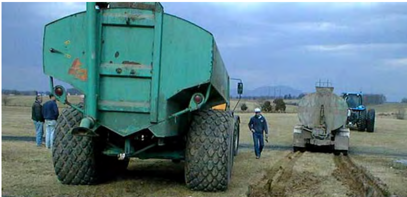
Fig. 3. Excessive rutting caused by narrow high pressure highway tires.
