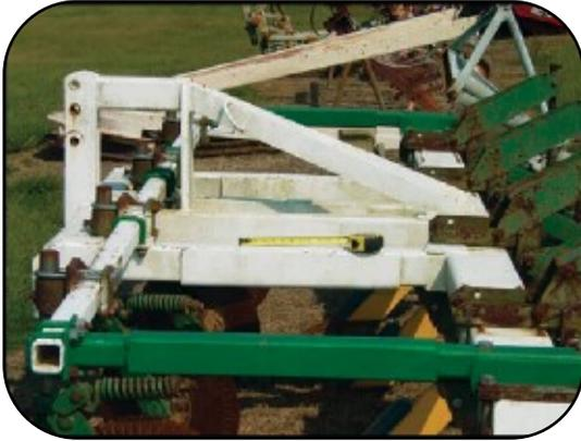
**Toolbar extensions** on older subsoilers can help ensure that the coulter is running on firm ground ahead of the shank to help cut residue.
