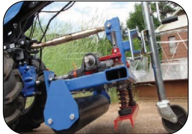
**Powered roller/crimper for walk-behind**
