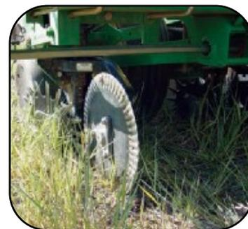
**Row cleaners** help move residue away from the seedbed to prevent hairpinning, which interferes with seed placement and can cause poor seed-to-soil contact. Row-cleaners should not be set too low or they will dig a trench into the seed bed.
