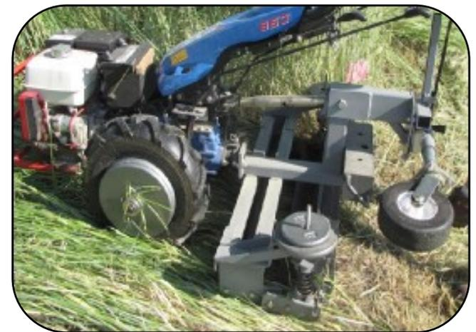
**Two-stage roller/crimper for walk-behind tractors**
