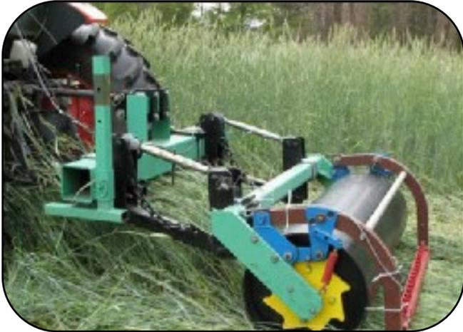
**Smooth roller with oscillating crimping bar assembly**
