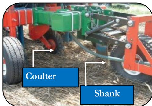
This is a modified one-row RJ Canadian made transplanter with an added sub-frame assembly to accommodate subsoil shanks and/or row cleaners. Combining subsoiling and transplanting operations eliminates the need for separate equipment, thus reducing labor needs and resources, such as fuel.
