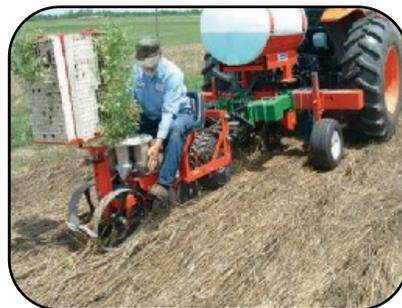
For greater stability, two driving wheels have been used, one wheel on each side of the crop row (instead of the original single wheel at the center of the row). This modification also helps minimize re-compaction of the soil opening created by the shank.
