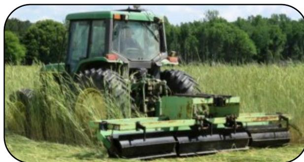
Straight crimping bar roller/crimper
