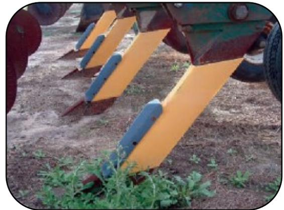
**Polyshields** help prevent soil build-up in heavy or wet soils.
