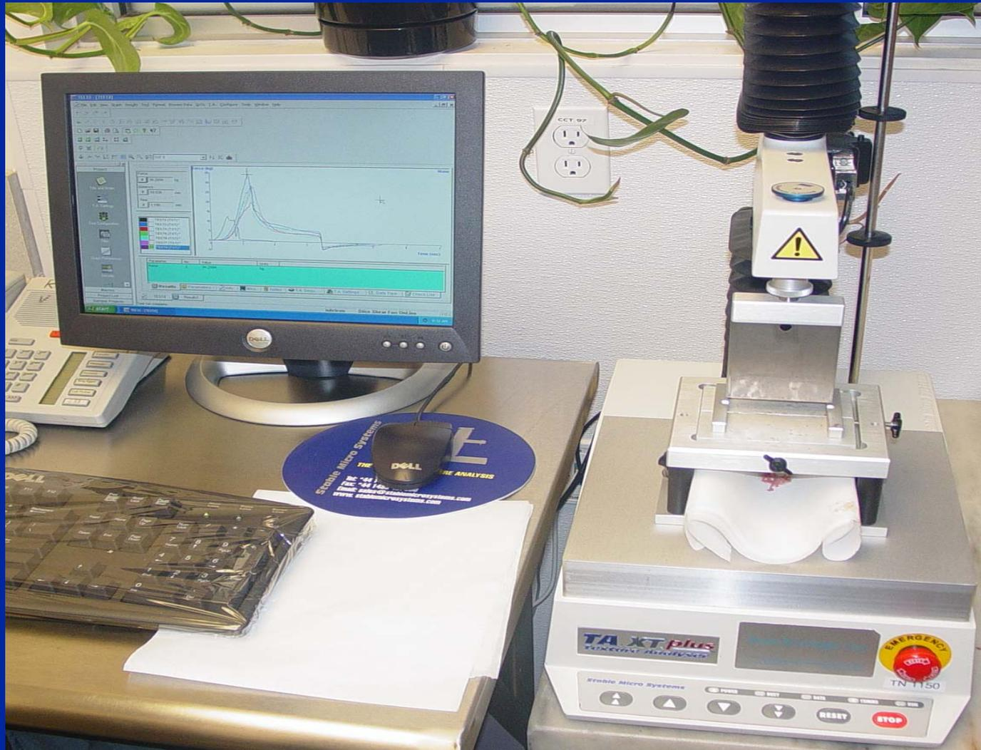
Shear the slice. The data should be captured by the instrument software on the computer running the instrument. We record the values as a backup for computer failure. The slot the blade passes through should be cleaned periodically with a paper clip. Rinse the slots the blade passes through with water periodically. The blade should be cycled through periodically with no slice to ensure the blade is free and not dragging.
