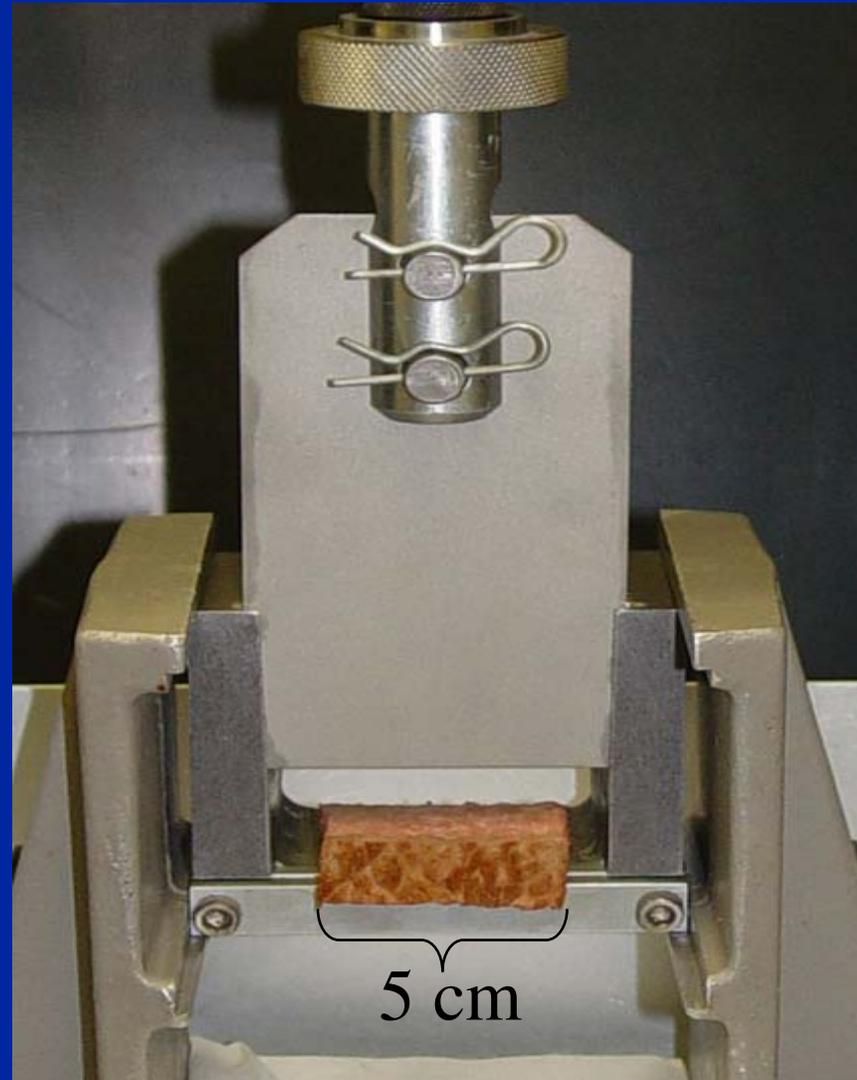
The slice blade should be 1.016 mm (0.04 inches) thick with the cutting edge beveled to a half-round. The spacers creating the gap for the cutting blade to slide through should be 2.0828 mm (0.082 inches) thick. The crosshead speed should be 500 mm/min for Universal Testing Machines (e.g., Instron, United, Texture Technologies, etc.).
