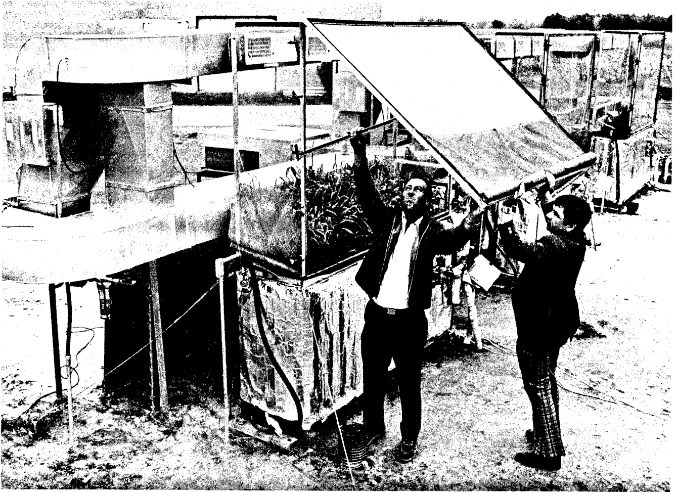
Top; Phene, right, and Jimmie Vought, hydrological technician, raise the clear side of a SPAR unit. Note the plastic shade on the side and two more units in the background. Left; Mary Fields, laboratory assistant, marks and dates root growth.
