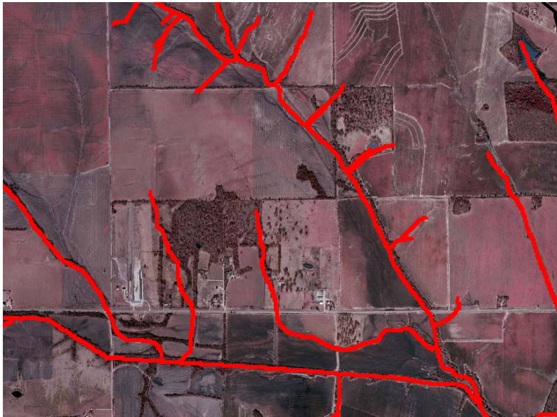
Figure 38 – A major confluence reflected properly by the generated stream network as indicated by the streams shown on the DOQQ.
