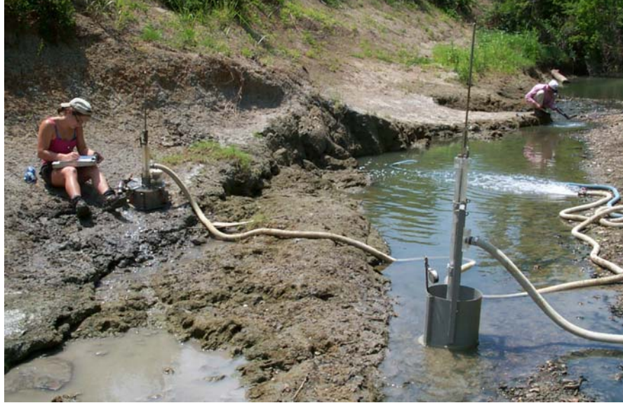
Figure 62 – Submerged jet-tests being conducted on the streambed of the main stem of James Creek. Vertical jet test device is in the foreground.
