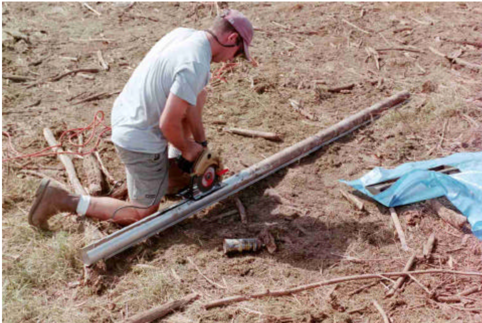
Figure 4-4. Photograph of extracted core being cut open on-site (June 1999).
