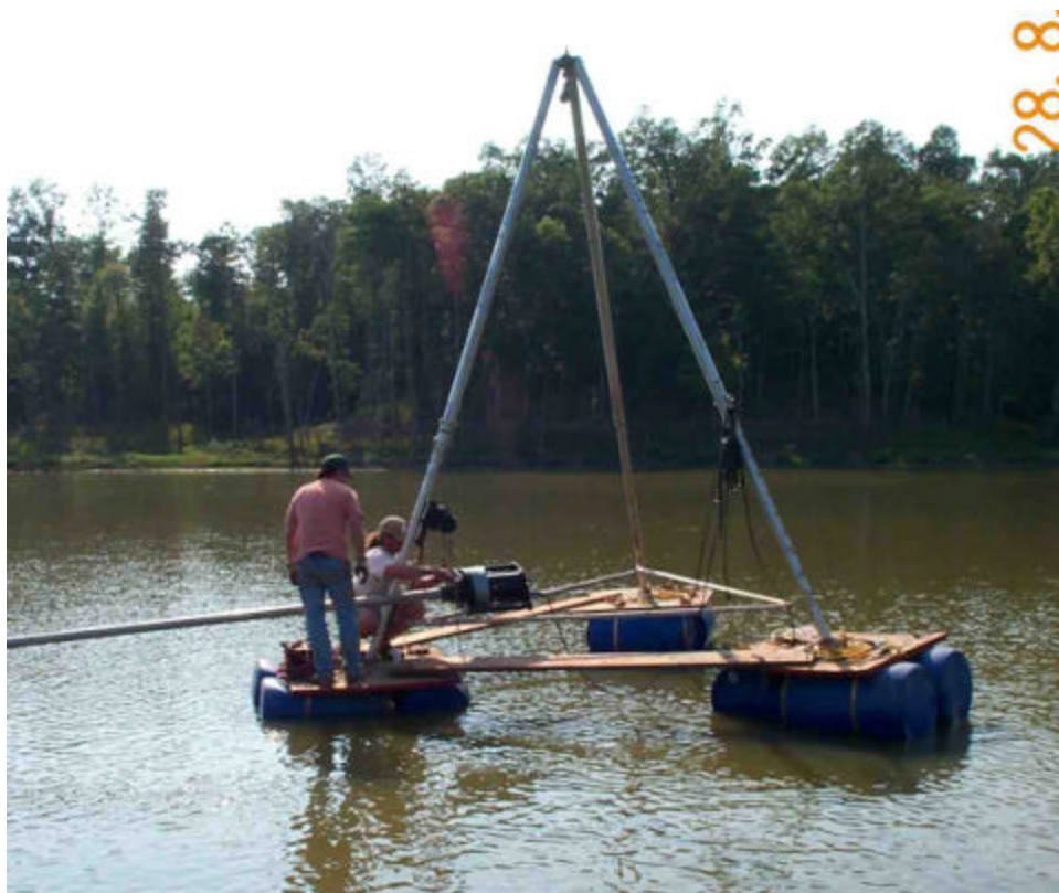
Figure 4-1. Photograph of floating vibracore system showing the tripod and portable rafts. A core pipe is being connected to the vibracore head.
