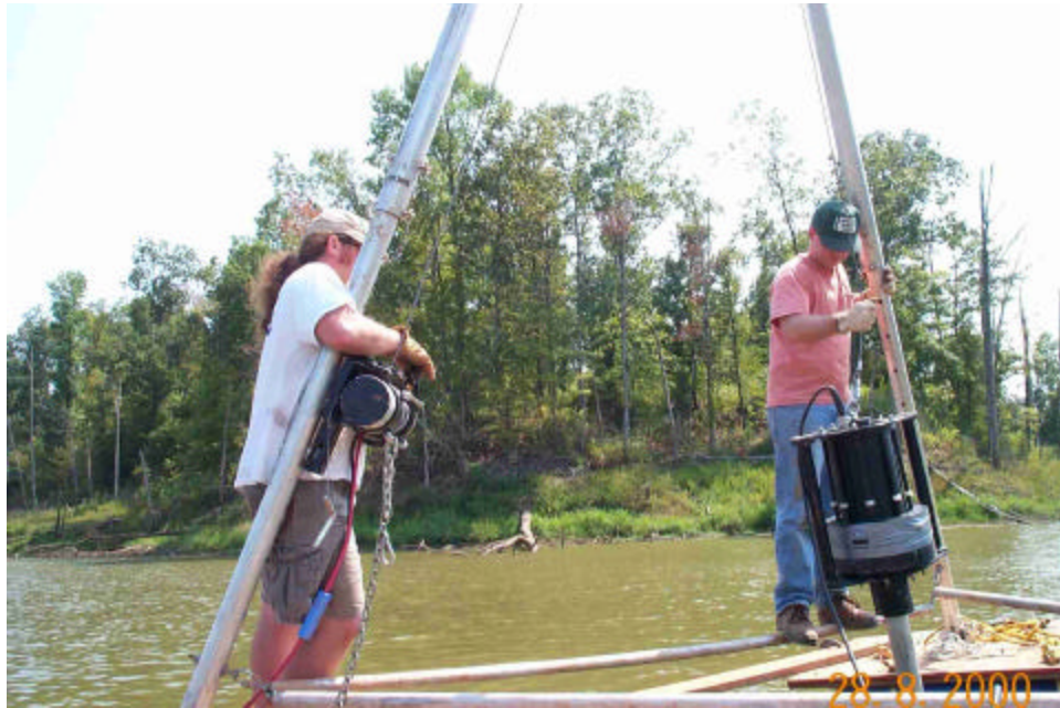
Figure 4-3. Photograph of vibracore system showing the tripod, vibracore head, and winch and cable assembly.
