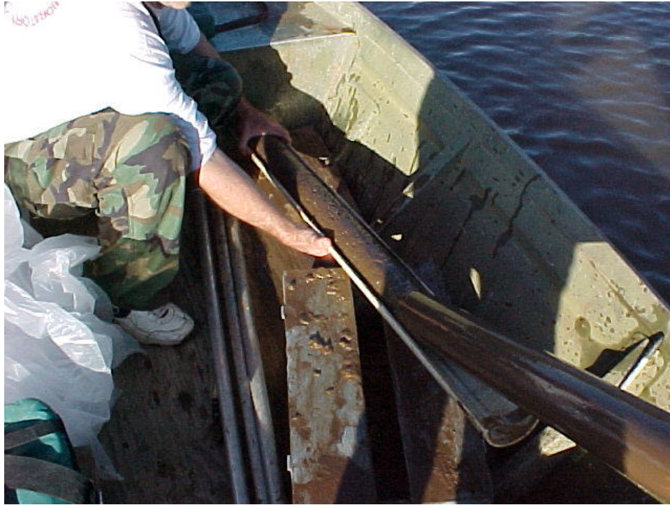
Figure 5-3. Photograph of the sediment core being extruded into core catcher (taken at Sugar Creek #12, October 1999). Core is extruded by tipping core and shaking out contents.
