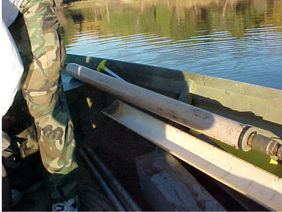
Figure 5-1. Photograph of the sediment coring tube used to obtain sediment samples (taken at Sugar Creek #12, October 1999).
