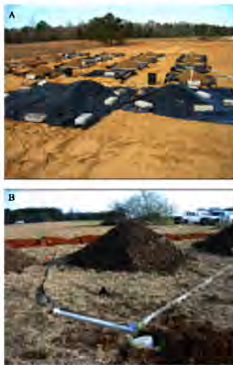
Fig. 1: Research sites: A) Research site with mini-piles of broiler litter and frames for collecting runoff, 2005; B) Research site with large boiler litter piles and flumes for collecting run off 2006
