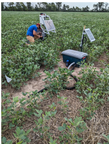
Data logger and soil moisture sensors being installed at various topsoil depths in the 88-acre soybean field.
