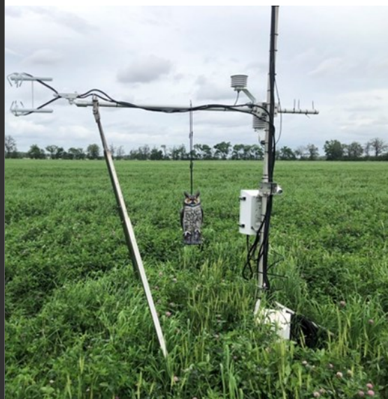
An eddy covariance tower used in this study to measure CO 2 exchanges between the atmosphere, soil, and crop.
