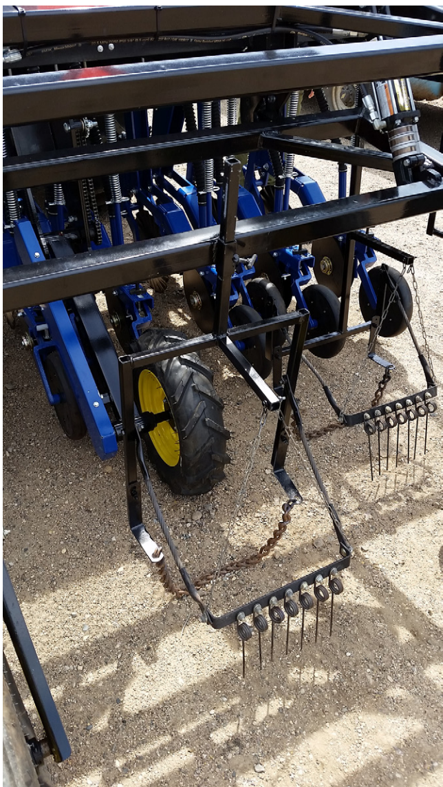
Fig. 1. Incorporation units consisting of a harrow-tine rake and light closing chain, installed with drill units lifted above the soil surface to simulate directed broadcast interseeding with light incorporation. Incorporation units were removed and the drill was lowered to achieve the high-clearance drill planting method.
