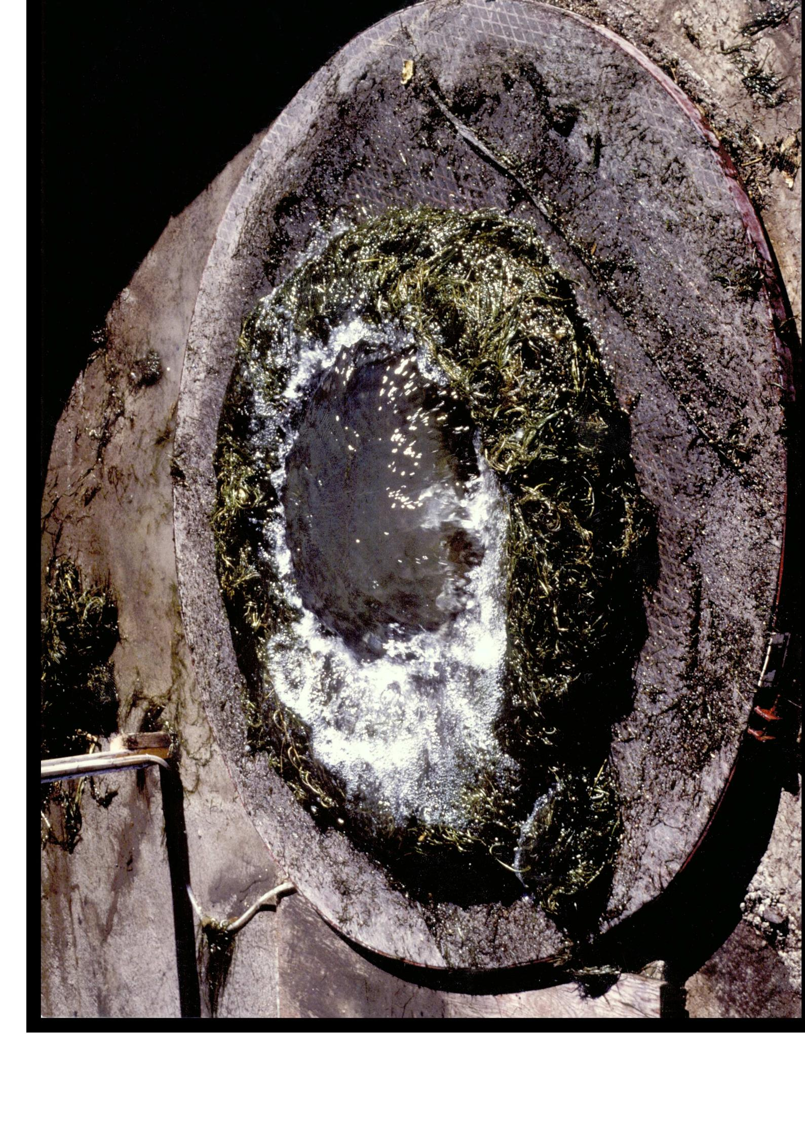
Pond weed accumulated on a bubbler screen. Pond weed is difficult to move off a screen. Perforated screen is smoother and works better with moss and pond weed.
